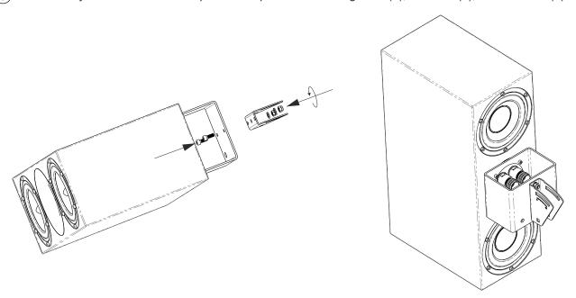
6 Slide speaker with mounting-assembly into place over wall-mount
