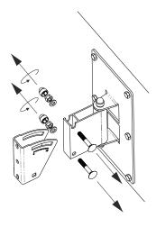
(5) Attach adjustable U-bracket to speaker adaptor-bracket using bolts (2), washers (2), and locknuts (2)
