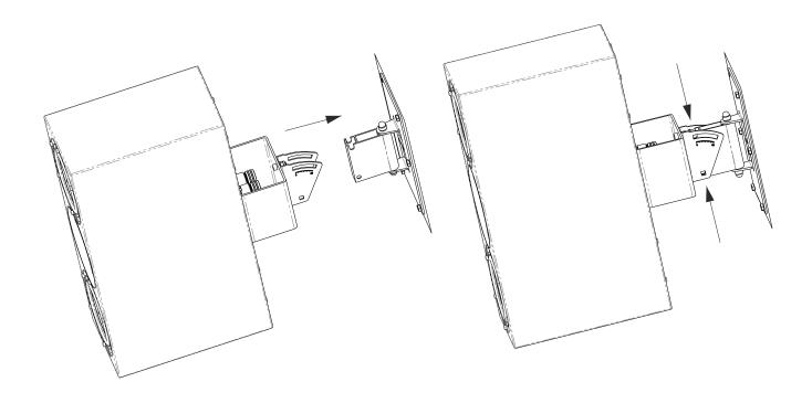
(7) Insert bolts (2), washers (2), locknuts (2), and locknut caps (2) to fasten adjustable U-bracket to wall-mount
