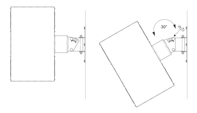
9 Adjust lateral monitor toe-in angle accordingly
