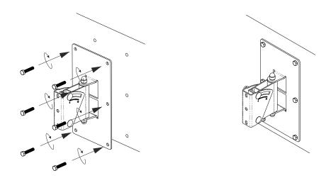
(4) Remove adjustable U-bracket from wall-mount ie. bolts (2), washers (2), locknuts (2), and locknut cap (2)
