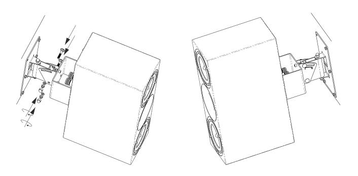
8 Set desired monitor tilt-angle (eg. 30 degrees pictured) and tighten adjustable hinge bolts
