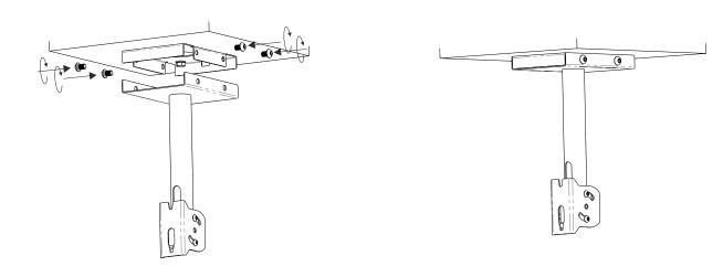
6 Slot lower mounting-post bracket to M6 bolts (2) on adaptor bracket and tighten
