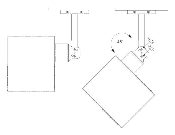
8 Adjust lateral monitor toe-in angle accordingly
