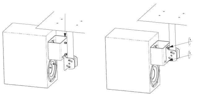
7 Set desired monitor tilt-angle (eg. 45 degrees pictured) and tighten adjustable hinge bolts
