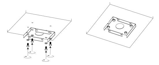
(5) Re-assemble mounting-post to base-plate with original bolts (4)
