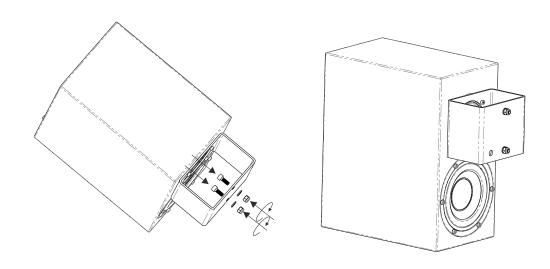
Mount base-plate of K&M bracket to pre-drilled/tapped ceiling panel with M4 bolts (4 bolts) and M6 washers (4)
