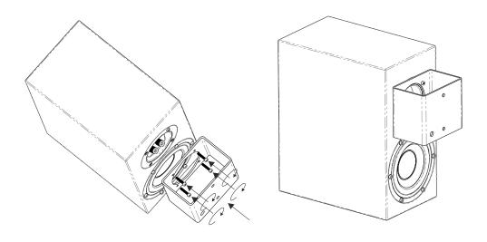
3 Loosely fit M6 bolts (2), M6 washers (2) and M6 locking nuts (2) to adaptor bracket
